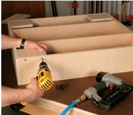
Add corner blocks. These provide strength and a solid place to attach the top with screws.
