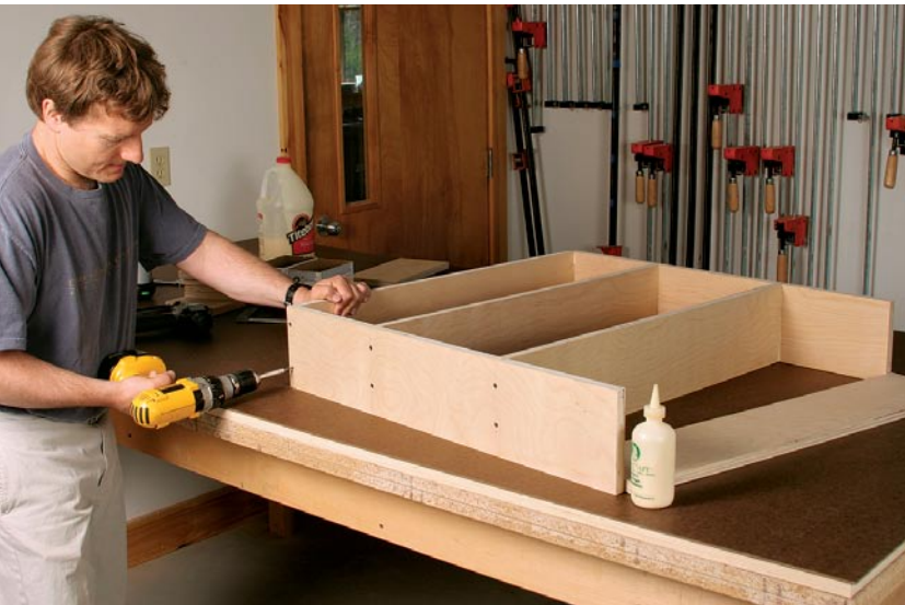
Glue and screw the sides and cross braces together. It's helpful to tack the pieces in place with brads first so they don't shift.
